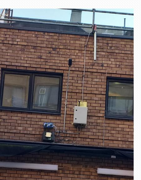
Microphone can be attached or mounted separately up to 10m away.
