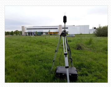
Deployed in pelicases, usually with a battery pack.
